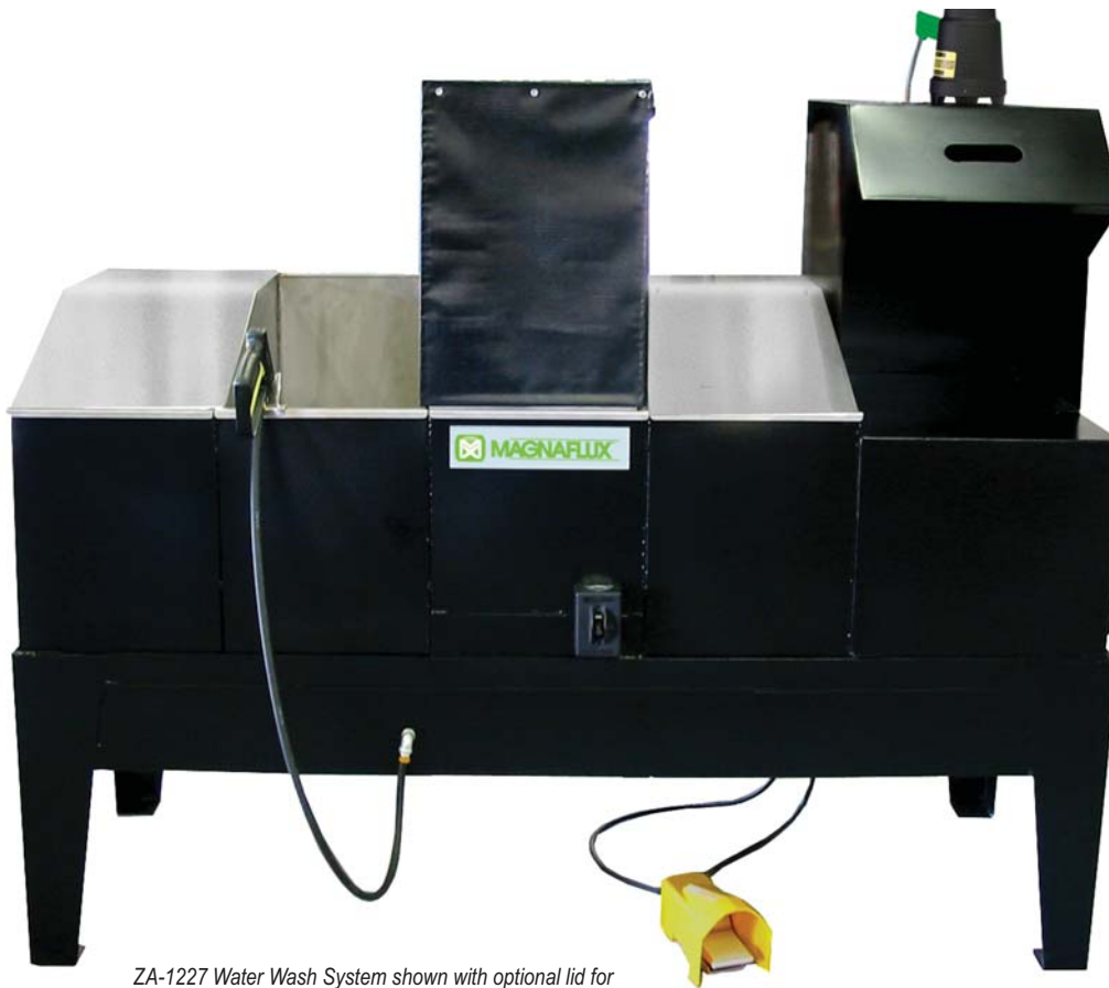
ZA-1227 Water Wash System shown with optional lid for penetrant tank and developer upgrade kit.
